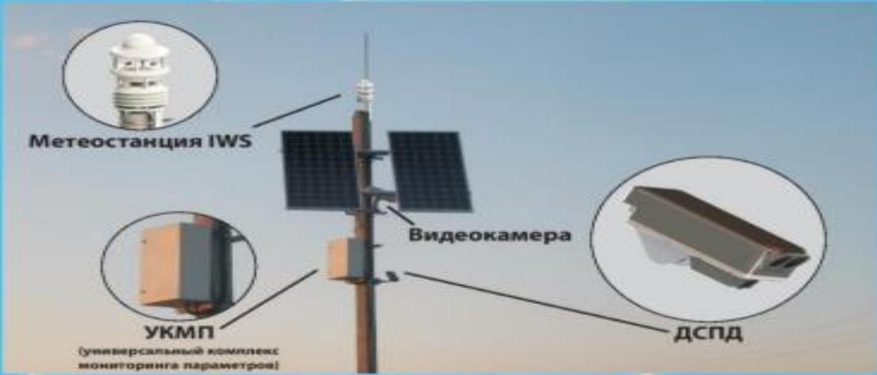
The diagram shows a central pole with several components: a weather station (IWS) at the top, two solar panels, a video camera, and a universal parameter monitoring complex (UKMP). Callouts provide detailed views of the IWS, UKMP, and a DSPD (Digital Signal Processor).
